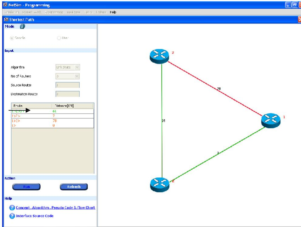
The screenshot shows the 'Shortest Path' window in NetSim. The network consists of three routers: Router 1 (top right), Router 2 (top left), and Router 3 (bottom center). The links and their distances are: Router 1 to Router 2 (78), Router 1 to Router 3 (7), and Router 2 to Router 3 (61). The shortest path from Router 1 to Router 3 is highlighted in green.
